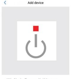
With all loads off, press and hold the power button for more than 6s and listen for two beeps.
