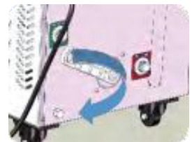
Close the lid with the plastic wrench
