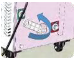
Open the lid with the built-in filter wrench.
