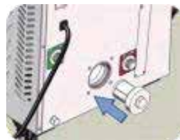
Put in the clean mesh filter.
